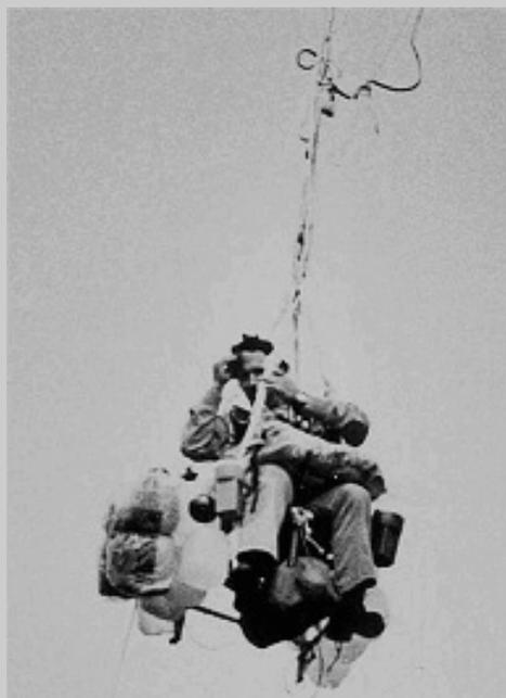
experiments with weights that he and his friends are reported to have conducted). Assuming a 4 foot radius each balloon would hold around 270 cubic feet of helium\* and thus generate a lift of over 14lbs (6.4kgs). So 40 or more of these would lift a man, chair and ballast without any problems! But lift is reduced by around 7.5% per 1000 feet, depending on the variations of both pressure and temperature with altitude. So, luckily for Larry, sooner or later he would stop rising...
